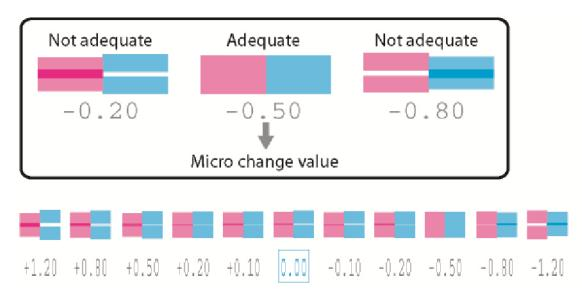
• After the micro adjustment printing is completed, "Micro Change: 0.00%" is displayed on Operation panel.
